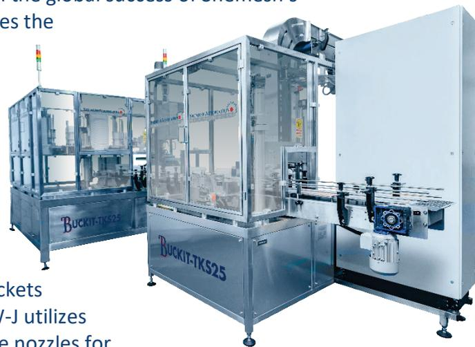
Packing up to 25 buckets per minute, the 'BuckIt TKS25' also includes the FGW-J buckets liquid filling and dosing machine. The FGW-J utilizes Shemesh-designed, height-adjustable wide nozzles for completely homogenous wetting of nonwoven rolls.
