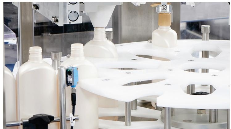
ETNA, the line's automatic bottle unscrambler, uses an ABB/FANUC spider robot to provide precise bottle orientation, covering virtually all bottle types common to the cosmetic sector. The robotic elements ensure no change parts are required (except in some cases for the robot grippers) when unscrambling multiple different bottle shapes. This results in much less downtime and a huge reduction in format parts costs over time.
