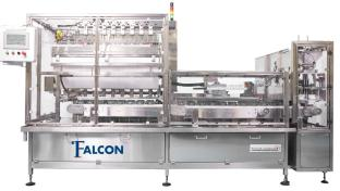
maximise the throughput from the denester. The Falcon filler handles problematic materials seamlessly and accurately. The tank and nozzles design guarantees that the liquid path is free from any kind of mechanical parts such as pistons and seals which can suffer from wear and tear because of the abrasiveness of certain materials."
