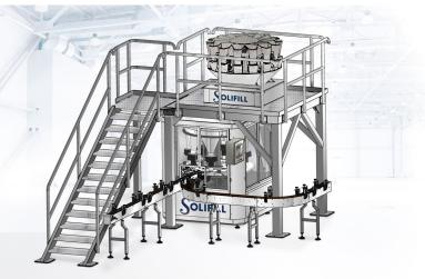
The bottles are fed through a timing screw into an infeed-starwheel which in turn feeds the main turret. Once in the main turret the combination scale filler is timed with the rotary platform to ensure accurate weight transfer. The product then travels onto a vibration section within the turret to allow for the transfer and settling of the entire dose into a narrow container / bottle opening.
