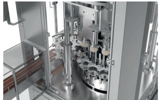
Rotary Piston Filling technology suitable for Viscous and Free flowing products
