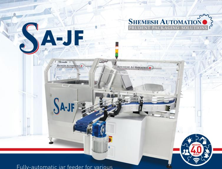
Fully-automatic jar feeder for various types of different shaped containers
