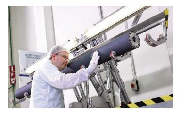
CFRP is becoming the material of choice for many applications in the nonwovens industry. Why? Critically, CFRP offers significantly reduced deflection over rollers made from other materials like steel and aluminum. This enables the use of much longer rollers, which in turn brings greater efficiency and larger scale to production, enabling greater sizes and faster speeds.
