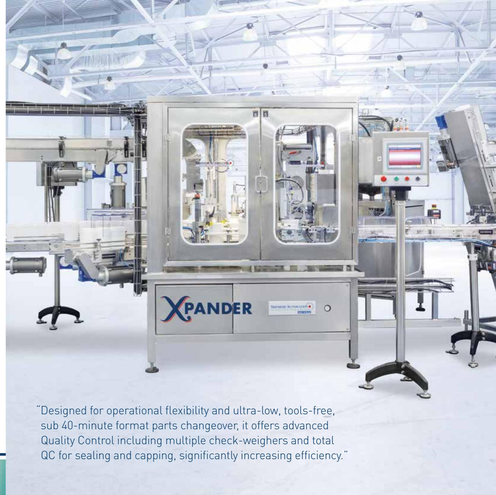
“Designed for operational flexibility and ultra-low, tools-free, sub 40-minute format parts changeover, it offers advanced Quality Control including multiple check-weighers and total QC for sealing and capping, significantly increasing efficiency.”
