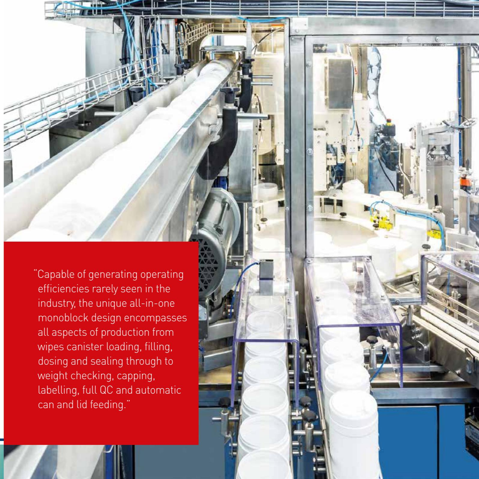
“Capable of generating operating efficiencies rarely seen in the industry, the unique all-in-one monoblock design encompasses all aspects of production from wiper canister loading, filling, dosing and sealing through to weight checking, capping, labelling, full QC and automatic can and lid feeding.”
