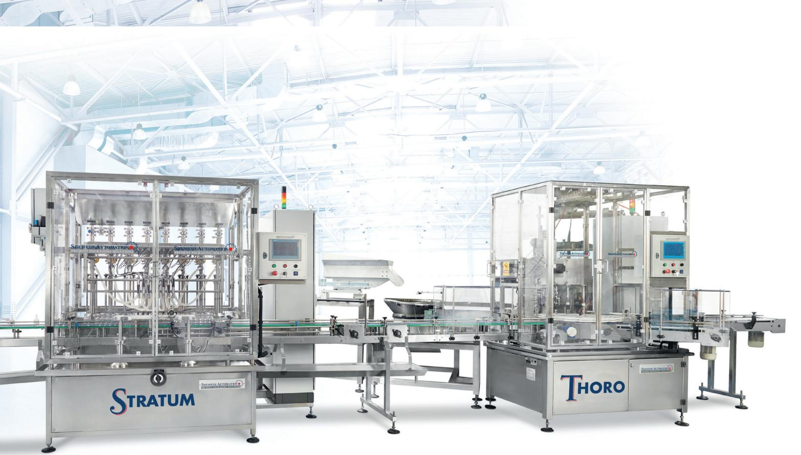
A fully integrated, Shemesh-made, automatic **STRATUM** filler & **THORO** capper basic line for gin. More advanced automation can also include automatic feeders, sealers, advanced QC, case packing and more – all under ONE umbrella and made by Shemesh.
