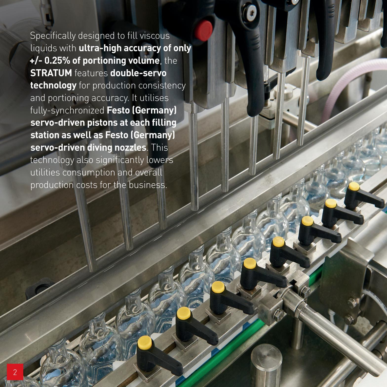
Specifically designed to fill viscous liquids with **ultra-high accuracy of only +/- 0.25% of portioning volume**, the **STRATUM** features **double-servo technology** for production consistency and portioning accuracy. It utilises fully-synchronized **Festo (Germany) servo-driven pistons at each filling station as well as Festo (Germany) servo-driven diving nozzles**. This technology also significantly lowers utilities consumption and overall production costs for the business.
