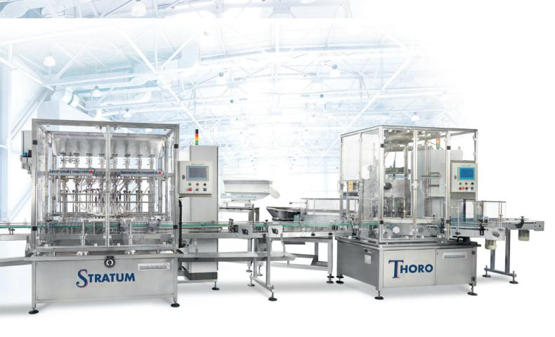
A fully integrated, Shemesh-made, automatic **STRATUM** filler & **THORO** capper basic line for gin. More advanced automation can also include automatic feeders, sealers, advanced QC, case packing and more – all under ONE umbrella and made by Shemesh.
