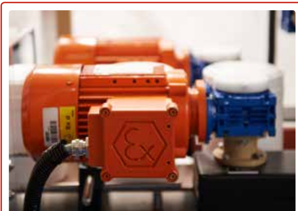
EX Approved Components such as SIEMENS motors, BANNER Sensors and SIEMENS PLC and HMIs
