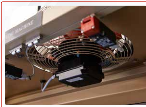
Built in ATEX rated commended ventilation systems for flammable fumes evacuation
